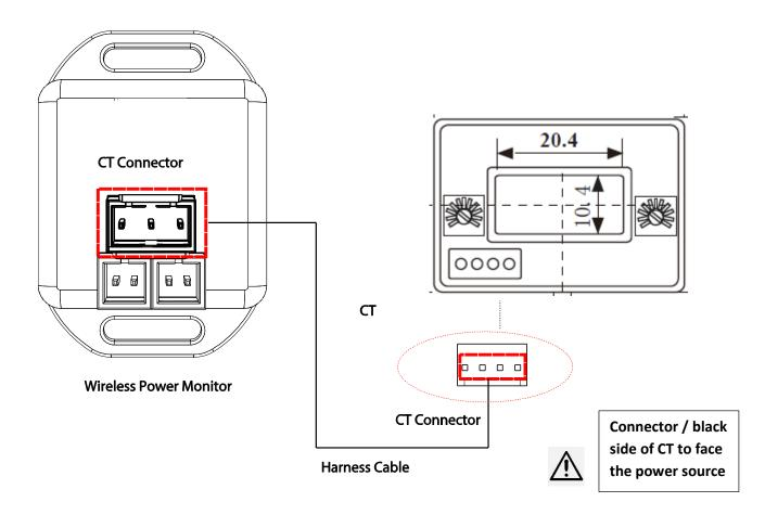
The arrow symbol on the top of the CT must point away from the power source and toward the load.
