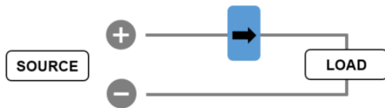
CT INSTALLED ON POSITIVE CONDUCTOR
