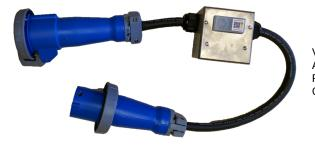
Voltage: 240V 3ØΔ Amperage: 20A Plug: IEC 60309 420P9W Connector: IEC 60309 420C9W
