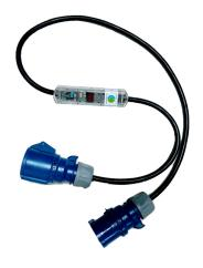
Voltage: 250V 1Ø Amperage: 16A Plug: IEC 60309 2P+E Connector: IEC 60309 2P+E
