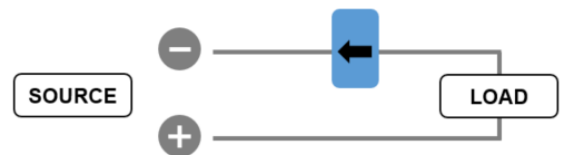
CT INSTALLED ON NEGATIVE CONDUCTOR
