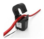
The side of the CT with the leads faces the source and away from the load.
