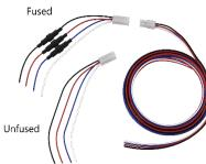
Voltage disconnects ("VDC") make it easy to stop power to the meter. The VDC consists of a 600V disconnect between two sets of 18 AWG 600V wire leads. Optional inline fuses are available on the meter (shorter) end. Can use either one or two VDCs (one for reference voltage and one for the meter's power source).
