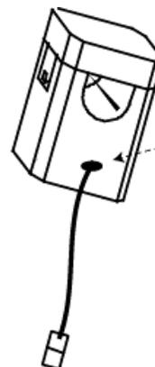
The side of the CT with the label faces the source and away from the load.
