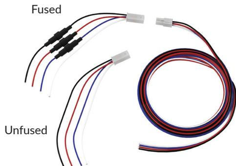
Voltage disconnects ("VDC") make it easy to stop power to the meter. The VDC consists of a 600V disconnect between two sets of 18 AWG 600V wire leads. Optional inline fuses are available on the meter (shorter) end. Can use either one or two VDCs (one for reference voltage and one for the meter's power source).
