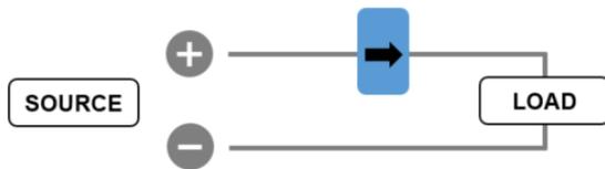
**CT INSTALLED ON NEGATIVE CONDUCTOR**
